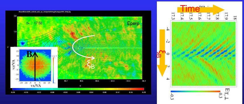
Temperature anisotropy  $(T_{e\perp}/T_{e\parallel} > 1)$  generates whistlers. Electrons are scattered to the parallel direction.
