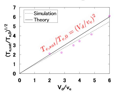
Wave amplitude saturates when the electron thermal velocity reaches the drift velocity, which is nearly equal to the phase velocity of the most unstable wave.
