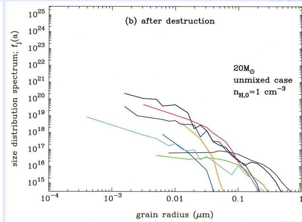
The size distribution of surviving dust is greatly deficient in small-sized grains, compared with that at its formation
