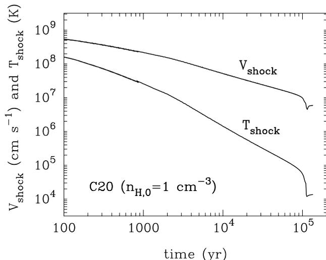
FIG. 4.—Time evolution of shock velocity  $V_{\text{shock}}$  and gas temperature  $T_{\text{shock}}$  at the shock front for model C20 with  $n_{\text{H},0} = 1 \text{ cm}^{-3}$ . [See the electronic edition of the *Journal* for a color version of this figure.]
