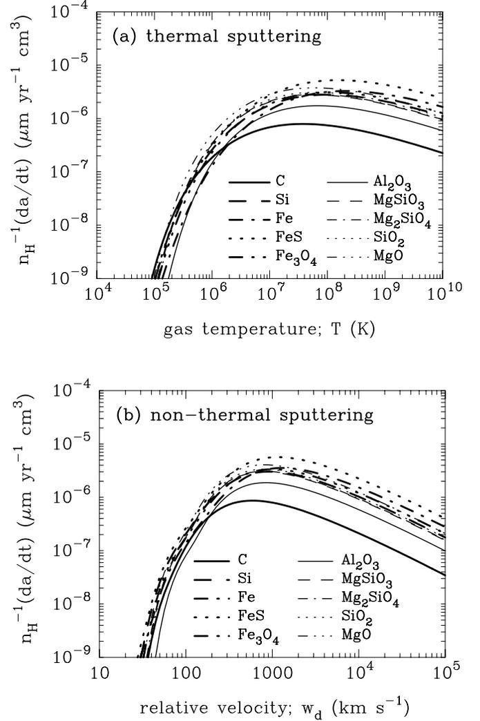
FIG. 2.—Erosion rate of each dust species by sputtering in units of  $\mu\text{m yr}^{-1} \text{cm}^3$  calculated for the elemental composition of gas with  $Z = 10^{-4} Z_\odot$  given in Table 1. (a) Thermal sputtering calculated by eq. (22) as a function of gas temperature  $T$ ; (b) nonthermal sputtering calculated by eq. (23) as a function of velocity of dust relative to gas  $w_d$ . [See the electronic edition of the Journal for a color version of this figure.]
