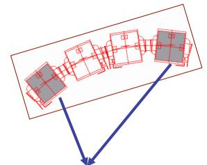
Outer 2 sector magnets are modified to achieve a precise isochronous field.
